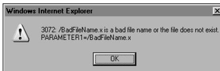
**Figure 2-6** Custom iServer error message for a missing file.
