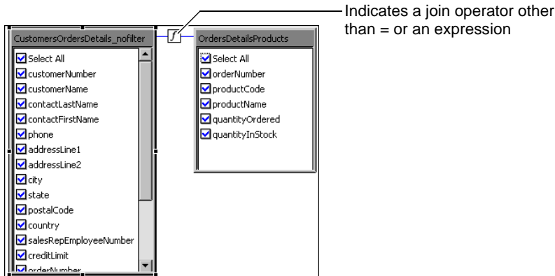
Figure 2-7 A join that uses an expression or an operator other than equality
